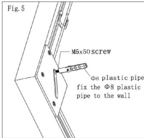
Insert the plastic pipe into the drywall and then hang the screen off the wall.
