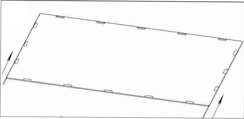
Carefully unroll the fabric, make sure the viewing side is placed on a clean surface to avoid getting the screen dirty. Place the four metal rods into the sleeves of material starting with the shorter sides first.
