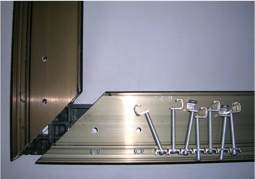
First unwrap screen material to determine how many tensioning screws need to go into the frame rails. You do this by looking at how many holes are on the sides of the screen material. Then insert the correct amount tensioning screws(F part) into the 4 frame pieces. Then insert 2 nuts(Part A) into each end of the longer frame piece and 1 nut into the each end of the shorter frame piece. Once completed it should look like the photo above.
