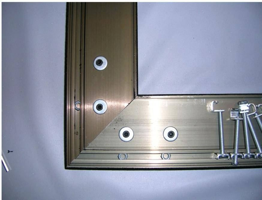
In this step, place all 4 frame pieces together, and then place part D and C into the 4 holes in each corner. Use part E to do so. After that is completed, it should look like the photo above.
